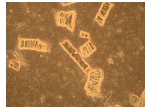
High throughput homogenizer with deep well plate and 5/32" grinding ball produced very fragmented muscle and a relative disruption efficiency of 52%.
